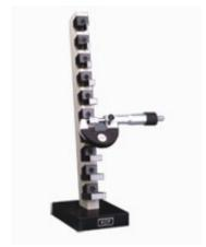
Best suitable for quick and reliable calibration of External Micrometer.
