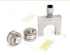
Air snaps are designed for those difficult to reach or "between centers" diameter measurements. Often, air snaps gage a part while it is engaged in the machine tool. Also Snap gages are ideal for production settings where specific diametrical or thickness measurements must be repeated frequently with precision and accuracy.
