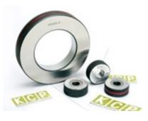
Ring Gauges are ideal for measuring outside diameter of work pieces. A ring gauge is also effective to check out of roundness on the higher side. A master setting ring is used as a standard to set bore gauges, which can then be used to determine deviation from the master size.
